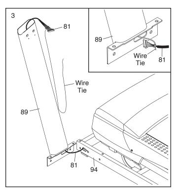
Hold the Left Upright (89) against the Base (94). Be careful not to pinch the Upright Wire (81). Insert two 3/8" x 1 1/4" Screws (8) with two 3/8" Star Washers (13) and two 3/8" x 2 3/4" Screws (7) into the Left Upright.
